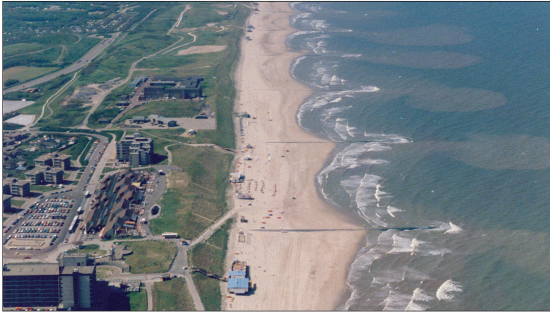
Figure 7: The groynes at Delfland Water Board: basalt groynes were built perpendicular to the coast to prevent the natural transport of sand along the coast. However, they have a negative impact because they initiate rip tides which transport sand away from the beach. Sand plumes result and literally and figuratively the coast is hollowed out.
