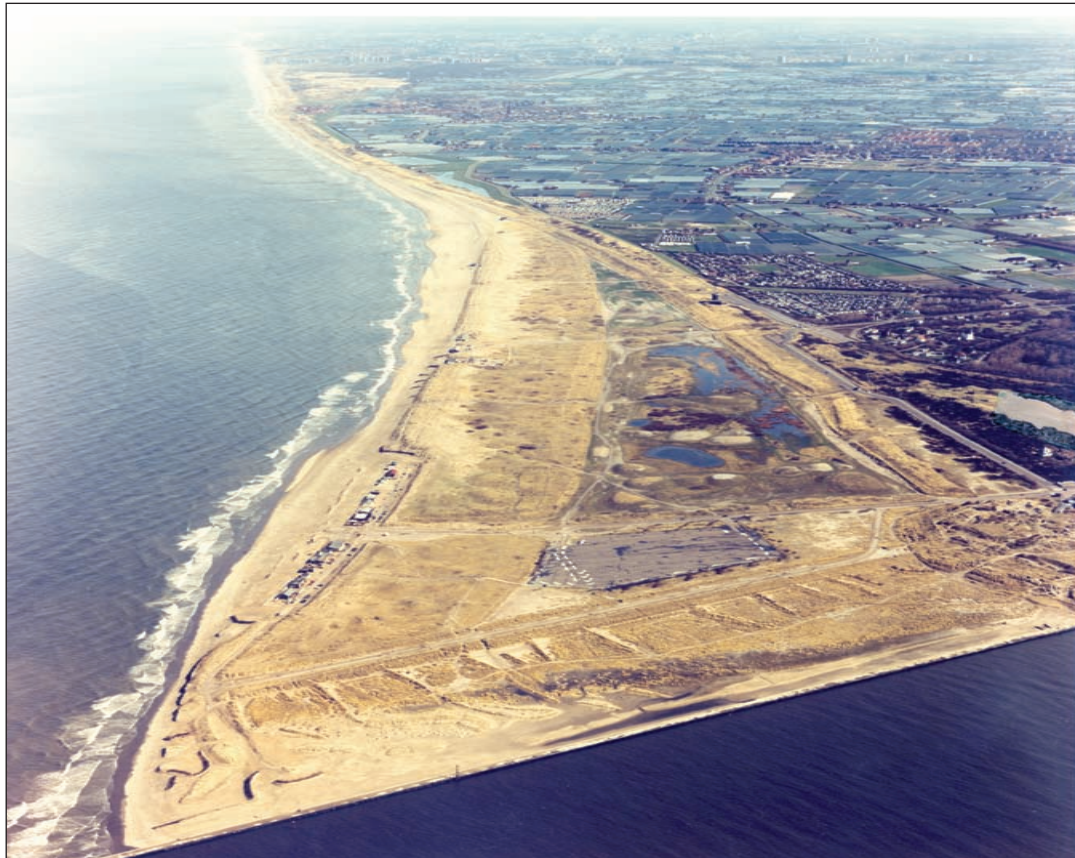
Figure 8: The first realised segment of Plan I from Hoek van Holland to Scheveningen, the so-called Van Dixhoorn Triangle, completed with a primary protective dune running parallel to a major thoroughfare in the Hague, the Laan van Meerdervoort. The coast orientation is good and 11 of the 68 Delfland groynes have disappeared under the sand. This is a land reclamation of ca. 150 ha with a splendid natural reserve, the Kapittel Dunes. South of this the train route Rotterdam to the Hoek van Holland will be lengthened and further roadways will be constructed, as well as 1100 homes and facilities. In the next phase a tidal lagoon will be realised for a yacht harbour and hotel conference centre, together with the already existing passenger-ship connection to the UK.
