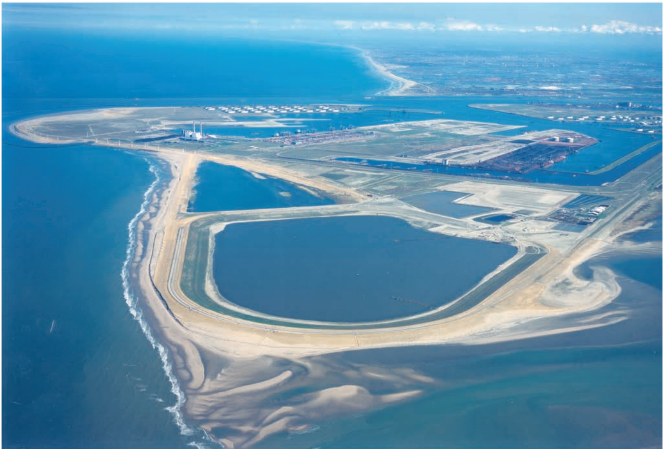
Figure 11: In the distance at the top of the photograph, the hollow Rhineland coastline – without any solid seawalls – can be seen. This coast has shown slight accretion since 1611. Where the hollow Rhineland coast meets the slightly convex attacked Delfland coast, the range of 68 Delfland Groynes commences. At the constructed Van Dixhoorn Triangle, north of Hoek van Holland 11 of these groynes are buried under sand and they are totally unnecessary. Below in front of and west of the motorway A15 the first 2 segments of Plan 2 are visible, with dunes and beach protecting them according to the principle of Building with Nature.
