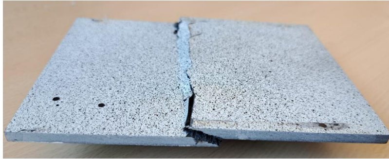
Figure 4: Failed specimen after CAI fatigue test.
