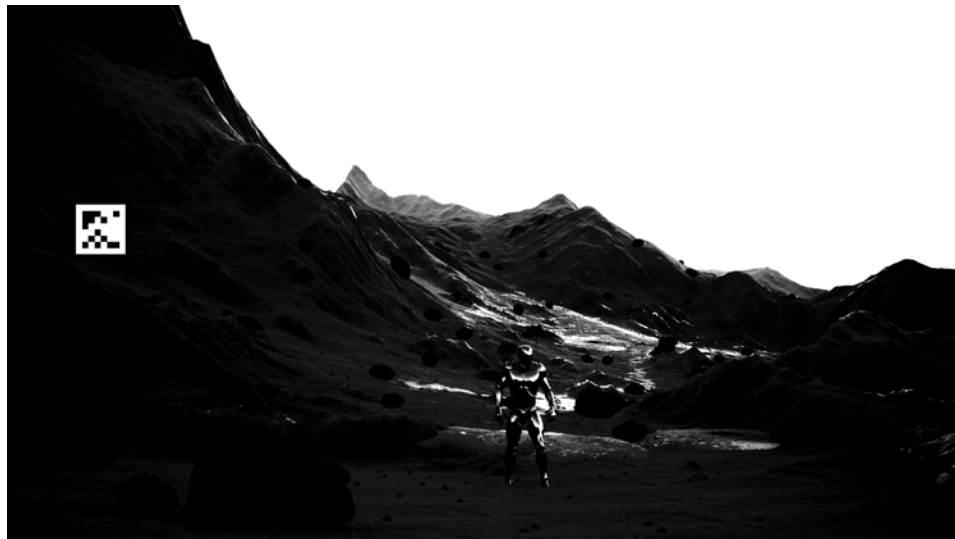
Figure 10: Case where OpenCV ARUco failed to find tags using 'aruco.detectMarkers' using default parameters.
